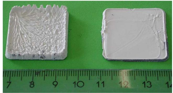
Fig. 7. Al<sub>2</sub>O<sub>3</sub> deposits obtained from MEK based suspensions containing 1 wt.% nitrocellulose and 2 (left) and 10 (right) vol% *n*-butylamine.
